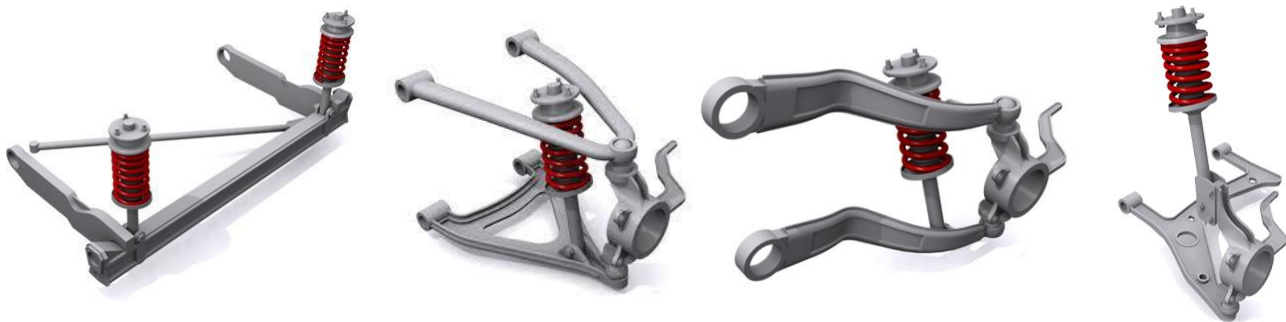
Twist Beam (Dependent) - Double Wishbone (SLA) - TriLink - MacPherson (Strut)
