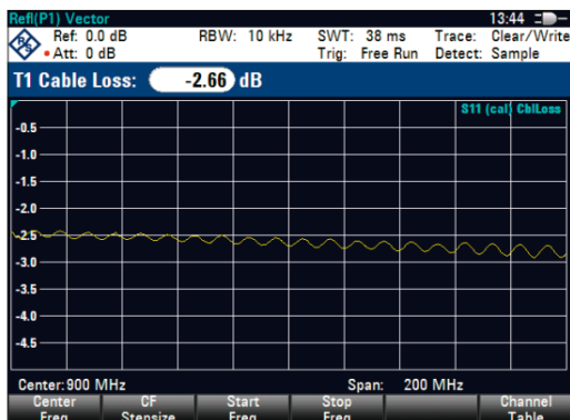
One-port cable loss measurement.
