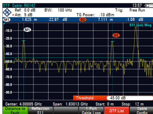
Distance-to-fault (DTF) measurement
