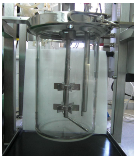
Figure 10: A. fermenter vessel mounted with one turbine DT6. B. fermenter vessel mounted with two turbines DT6 – DT6.
