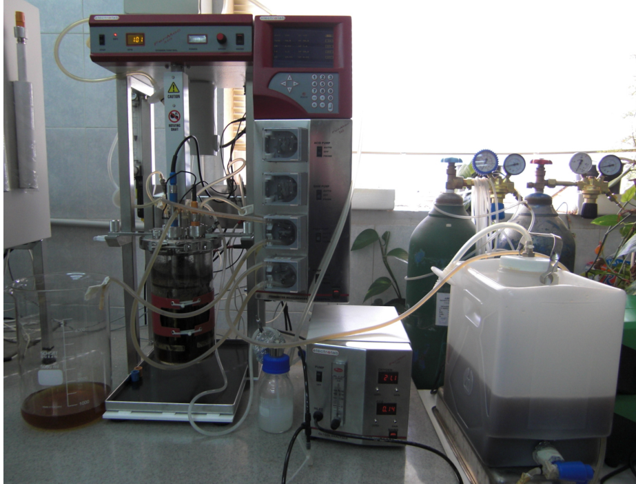
Figure11: xylanase production during continuous culture of Aspergillus niger in a 3-L bioreactor fitted with two DT6.
