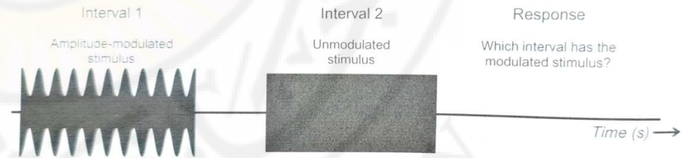
FIGURE 5-11. Illustration of an experimental trial for a modulation detection task. Here, the modulated stimulus has 50% amplitude modulation (a modulation depth of 0.5).
