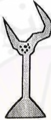
الشكل (١٣ - ٢٣) Shrink - spot porosity - Sprue attachment too bulky. Sprue too long or thin. Button too small.
