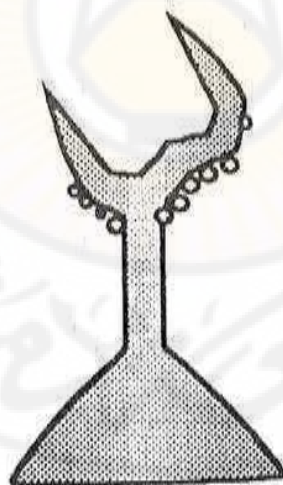
الشكل (١٣ - ٢٢) Nodules on one side only - Prolonged vibration after pouring
