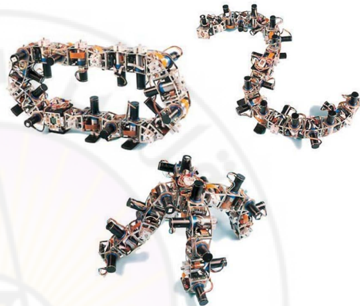
Figure 7.2. Robotic modules can be reconfigured to "morph" into different locomotion systems including a wheel-like rolling system (left), a snake-like undulatory locomotion system (right), a four-legged walking system (bottom).
