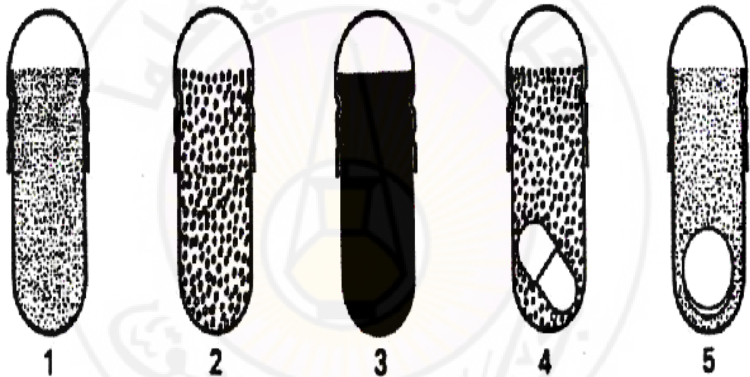
FIGURE 7.8 Examples of fill in hard gelatin capsules. 1, powder or granulate; 2, pellet mixture; 3, paste; 4, capsule; and 5, tablet. (Courtesy of Capsugel Division, Warner-Lambert.)
