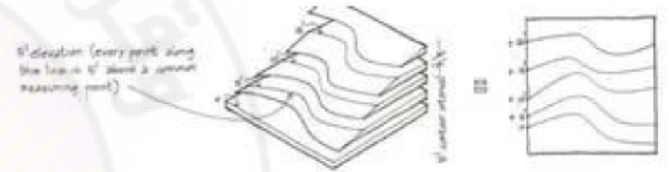
Relationship between 2-D and 3-D representation of site topography (contour lines)
