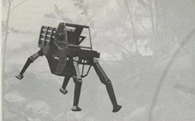
The walking truck, a unique means for locomotion over off-the-road terrain, utilizes a "force feedback" control system thereby creating a cybernetic man-machine relationship. A research prototype has proven the feasibility of the quadruped machine.
