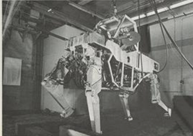
The walking truck, a unique means for locomotion over off-the-road terrain, utilizes a "force feedback" control system thereby creating a cybernetic man-machine relationship. A research prototype has proven the feasibility of the quadruped machine.
