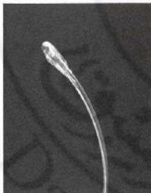
FIGURE 4.2. Photograph of tympanic membrane electrode (the gel-covered silver wire at the end of the electrode that makes contact with the tympanic membrane).
