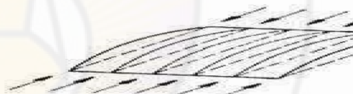
a) column-like beh of plates without longitudinal sup
